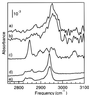
**Figure 1.** Unpolarized infrared spectra of cyclopentene on C(001), Si(001), and Ge(001) surfaces. (a) Spectrum of C(001) after exposure to 10 000 langmuirs of cyclopentene, 300K. (b) Spectrum of C(001) after exposure to 20 000 Langmuirs of cyclopentene, 300 K. (c) Spectrum of cyclopentene multilayer condensed onto C(001) surface at 90 K. (d) Spectrum of Si(001) after exposure to 10 langmuirs of cyclopentene, 300 K. (e) Spectrum of Ge(001) after exposure to 10 langmuirs of cyclopentene, 300 K.
